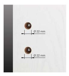
Door preparation for HOPPE handle sets on mini-rose with emergency release and turn for bathroom/WC doors
